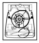
freely, it also should be removed for cleaning. To remove the fan, place a wrench over the motor pulley. Hold the fan blades with one hand and turn the wrench counterclockwise. Remove the motor pulley and lift the fan off the motor shaft. Clean the area and replace the fan over the motor shaft. Tighten the motor pulley snugly clockwise with the wrench. If necessary, replace the fan cover or the gasket with replacement parts.
